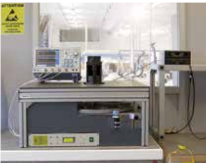
Custom made Jig for optical encoders dynamic tests.
